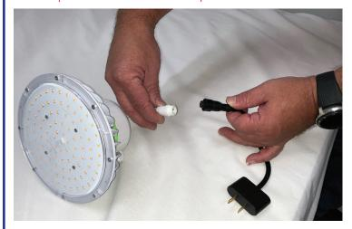
Step-3: Secure the Connection by Tightening Nut on HL-LS-GX16D Adaptor
